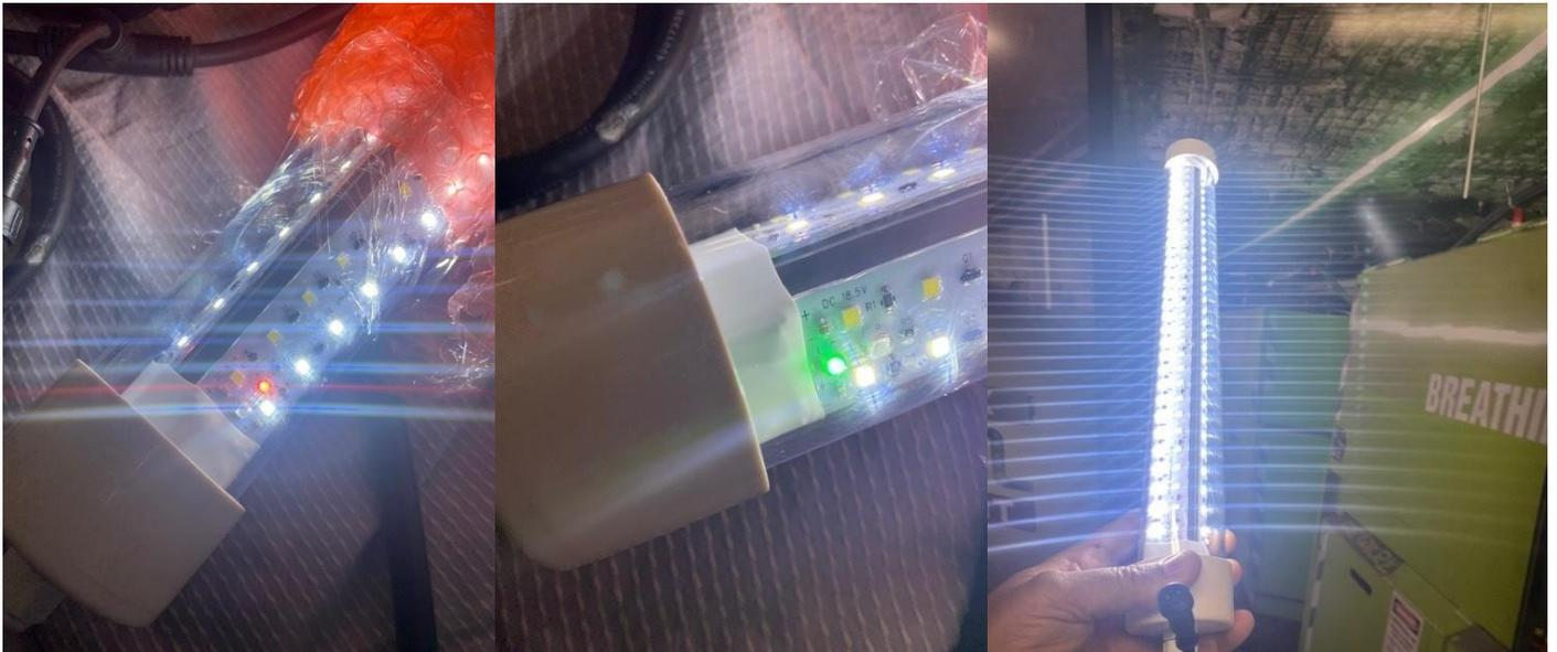
When charging the light is on, and the indicator is red. When fully charged the indicator will turn green. Once charged the emergency light will run for up to 4 hours.
